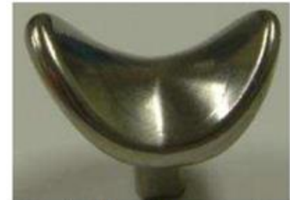
The artificial finger joint prototype made of Ti-based metallic glass. The saddle-shaped structure on the upper side is a
